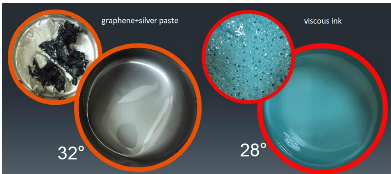
Figure 2 High-precision mixing results: The image demonstrates the effectiveness of blade-free vacuum planetary mixing in achieving uniform consistency. On the left, graphene-silver paste is thoroughly homogenized, reducing air pockets and enhancing material integrity. On the right, viscous ink shows significant deaeration, ensuring a smooth, defect-free final product. Temperature measurements indicate efficient heat dissipation during the mixing process.
