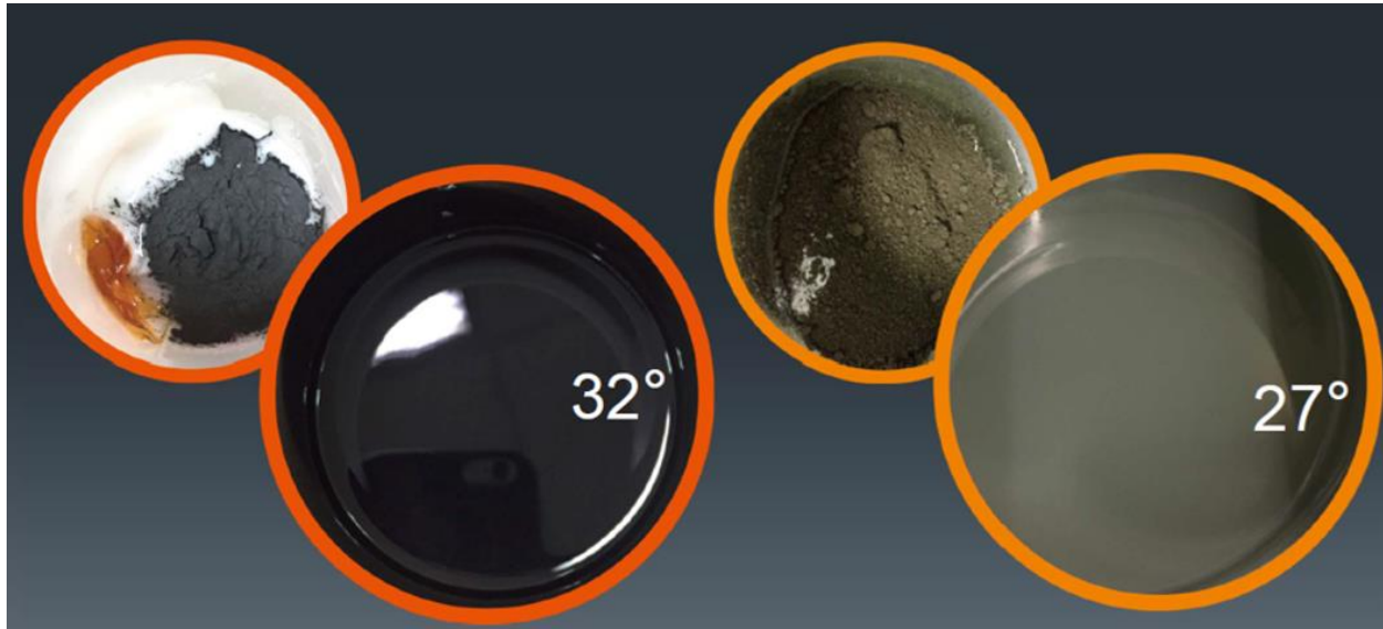
Figure 3. Comparison of mixing results for high-viscosity materials using a blade-free vacuum planetary mixer. The left side shows a high-density metal powder (SENSOR layer) mixed at 8,000–10,000 CPS viscosity for 4 minutes, achieving a uniform and smooth consistency with a final temperature of 32°C. The right side demonstrates binder and nickel oxide powder (fuel cell anode substrate) mixed at 5,000–6,000 CPS viscosity for 3 minutes, resulting in a well-dispersed mixture with a final temperature of 27°C. The vacuum mixing process ensures superior homogeneity and effective deaeration.
